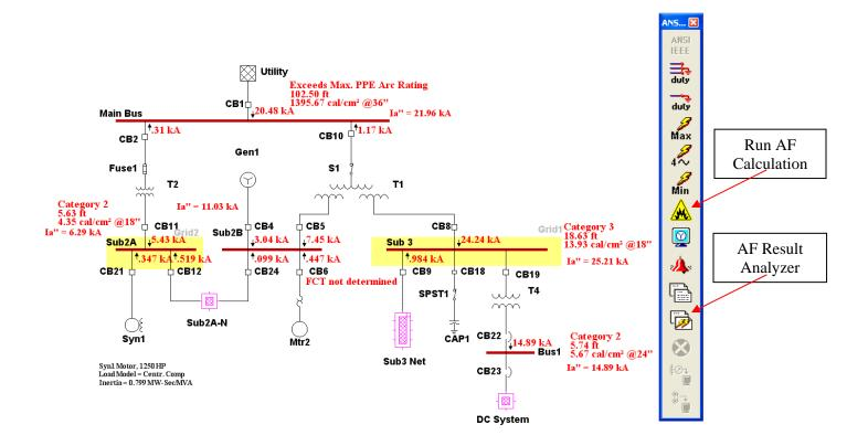
The AF calculations can be repeated for all the different configurations in ETAP. The Scenario and Study Wizards can be used to keep track and repeat the different calculations as shown in the images below where two different AF calculations were performed and recorded:
