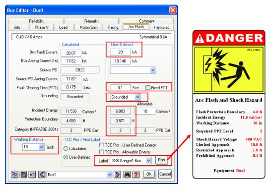
Select the arc flash label template that you want and click on the Print button. A Crystal Reports viewer window will open with a label that is ready for printing. The bus Arc Flash page allows you to get Arc Flash results instantly.
