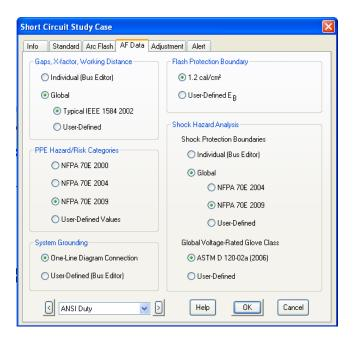
The global definitions for each set of input data parameters can be modified or reviewed by accessing the Project \ Settings \ Arc Flash \ menus as shown below:
