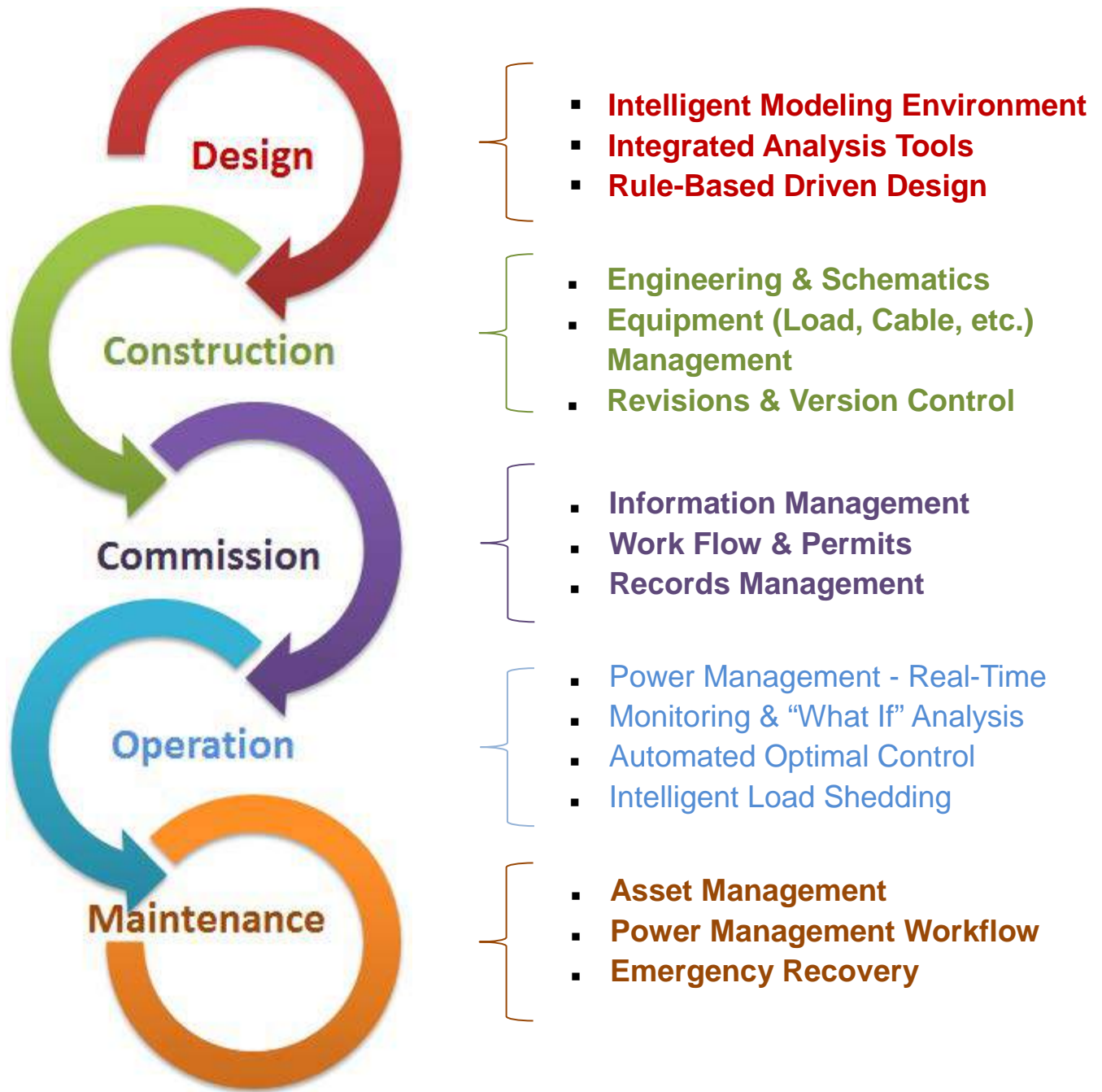
Figure 3: The electrical distribution system life cycle covers five main phases.
