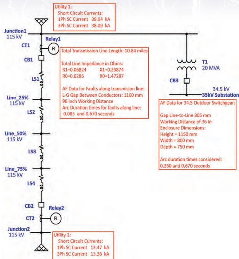
**Figure 8:** 115 kV Transmission System One-Line Diagram
