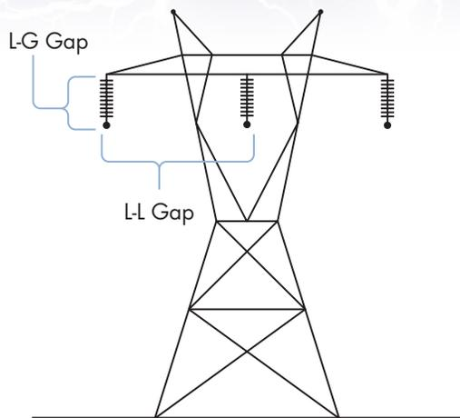
**Figure 6:** 120 kV Transmission Line Design
