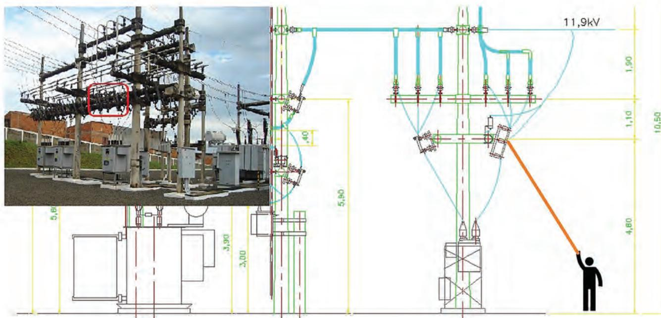
**Figure 3:** *Outdoor Substation*
