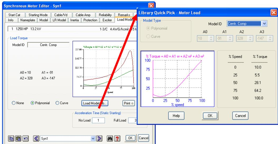
Also, go to the Inertia page and enter 0.2 into the motor inertia (H) field, and click OK. The motor  $WR^2$  will automatically be updated. Exit the Syn1 Synchronous Motor editor by clicking OK.
