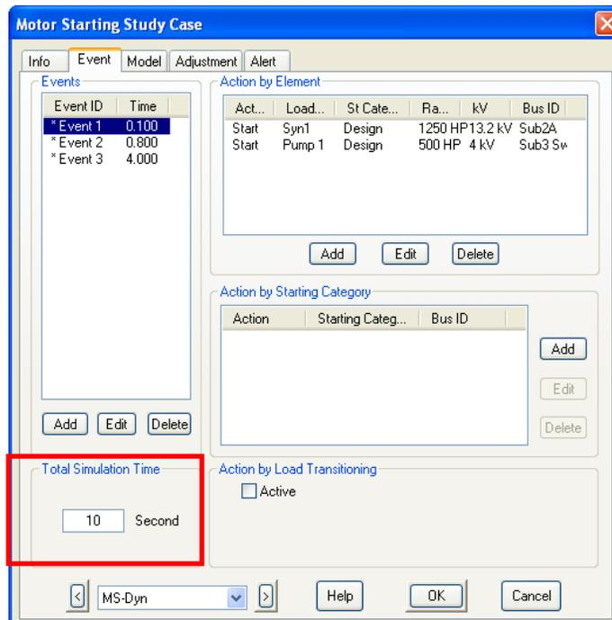
Now you can add an unlimited number of events to simulate switching actions in a single Motor Starting simulation. You can start or switch off individual loads or categorized motor groups with the Action by Load and Action by Starting Category features, respectively. You can also change the operating load by clicking the Load Transitioning option to change from one loading category to another.
