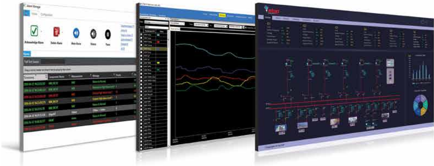
Electrical SCADA Human Machine Interface templates
