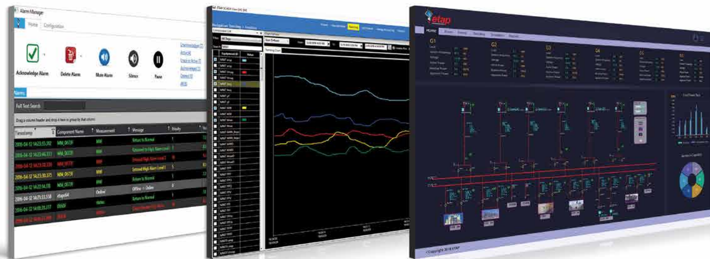
Electrical SCADA Human Machine Interface templates
