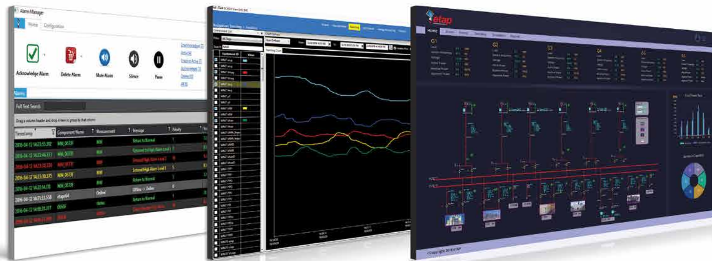
Electrical SCADA Human Machine Interface templates
